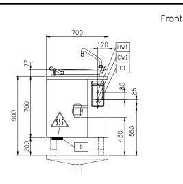
CWI1 = Cold Water inlet 1 (cleaning) Electrical inlet (power) Hot water inlet
